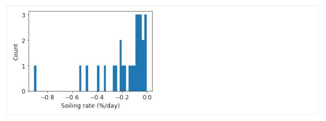
These plots show generally good results from the SRR method. In this example, we have slightly overestimated the soiling loss because we used the default behavior of the method key word argument in rdtools. soiling\_srr(), which does not assume that every cleaning is perfect but the example artificial soiling signal did include perfect cleaning. We encourage you to adjust the options of rdtools.soiling\_srr() for your application.
