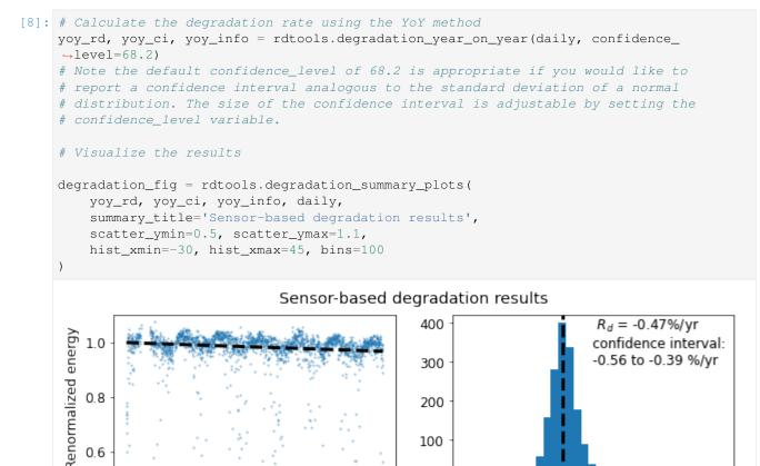
In addition to the confidence interval, the year-on-year method yields an exceedance value (e.g. P95), the degradation rate that was exceeded (slower degradation) with a given probability level. The probability level is set via the
