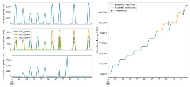
Examining the plot of estimated lost power, we can see that the estimated loss is roughly in proportion to the amount of offline capacity. In particular, the loss estimate is robust to mixed outage and communication interruption like on the 5th when only the smallest inverter is reporting production but the analysis correctly inferred that one of the other inverters is producing but not communicating.
